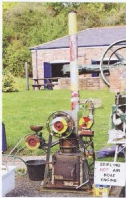
Malcolm Rowney brought along a rhombic-drive hot-air engine used to propel small boats, typically 12 to 16 feet in length.
