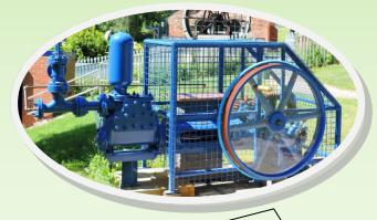
How does the turning of the wheel become reciprocating (back-and forth) motion to move the piston? What is the mechanism called? Is there one in a car engine?
