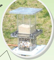
It is the fine sand which filters the water. So what are the pebbles, small stones and large stones underneath the sand for?
