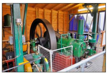
Outside the main building, the single-cylinder Wilson Oil Engine powered the Massington Lineshaft.
