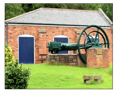
Horizontal steam engines were used to provide power in 19th century mills and factories. One engine could drive many looms or machines by the use of overhead line shafts and belts.
