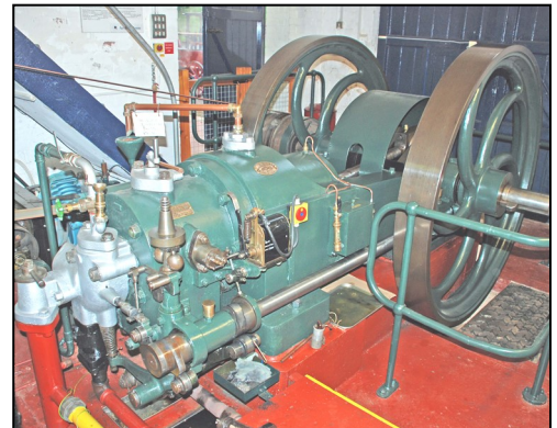
National gas engine installed in 1912 to replace two steam cylinders for driving the Joseph Evans' pumps through a gear box
