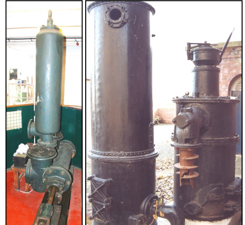
One of two Joseph Evans' pumps 1886 (left) and the producer gas plant (1912) which powered the National gas engine
