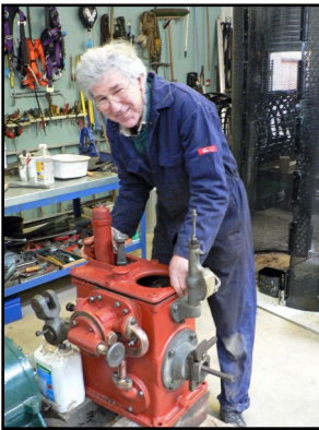
Maintenance on the water turbine's regulator in 2010
